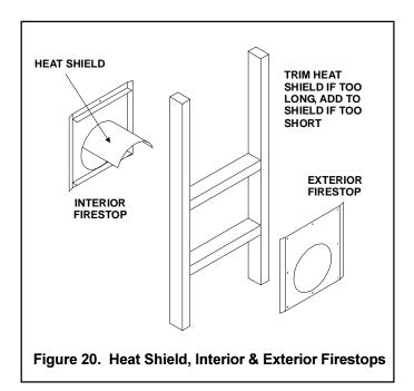
**For Vertical Runs -** One ceiling firestop is **REQUIRED** at the hole in each ceiling through which the vent passes.
